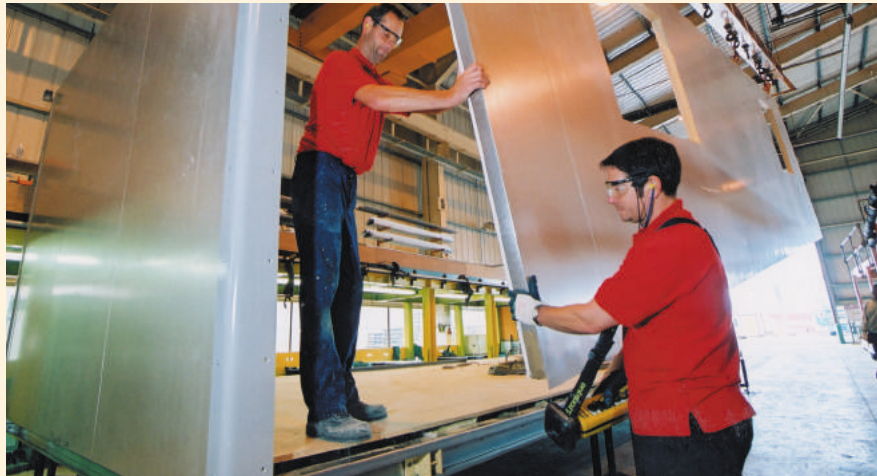
Steel framed room modules are manufactured and fully fitted out in a British factory
